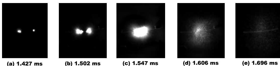
Figure 5.7(a)-(e) Images during the combustion of Al-Sb 2 O 3 . The time stamps shown below each frame correspond to the time from the start of the heating pulse.
